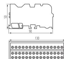
Terminal block is used for power distribution, it is adapted to cable lugs.
